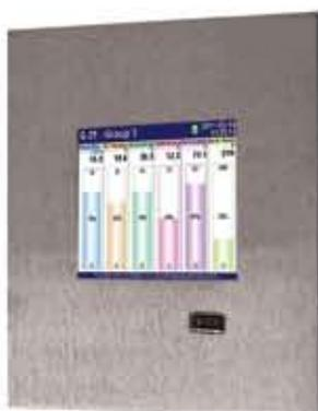
**Panel mount MultiCon ATG-500** is featured by a shallow casing – only 50 mm! All connectors are introduced on side walls of the device as in a typical panel computer. As the number of measurement inputs and outputs is limited, this design is intended mainly for systems with a small number of signals or systems which include other measurement systems with Modbus RTU interface. An Ethernet interface is also available to upgrade every MultiCon control's application easily.
